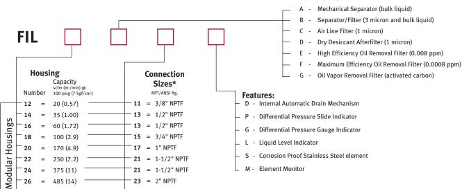
Example 1: To order a Grade E High Efficiency Oil Removal filter with a capacity of 100 scfm and 3/4" NPTF connections, integral automatic drain, differential pressure gauge, and liquid level indicator would be configured as: FIL18E15DGL
